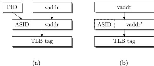
Figure 2: Tagging of TLB entries with (a) hardware supported and (b) emulated ASIDs.
