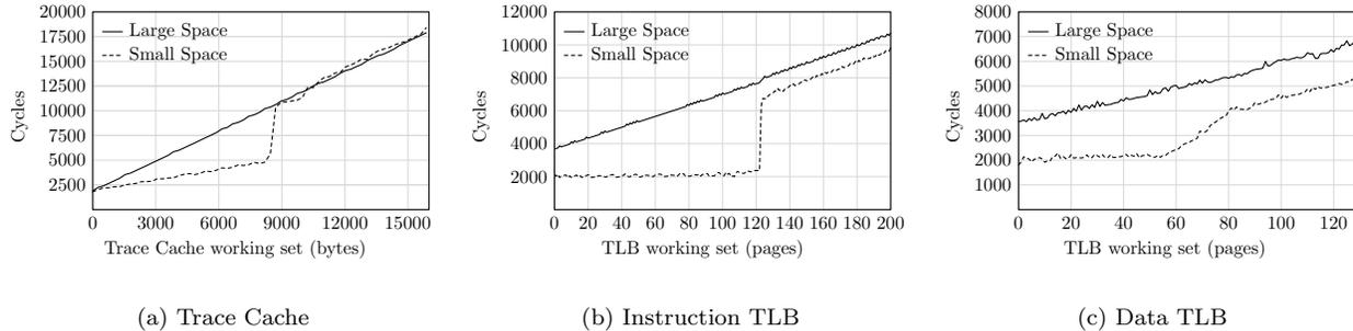
Figure 4: Execution time per IPC round trip (averaged over 100 executions) as a function of the trace cache and TLB working sets.
