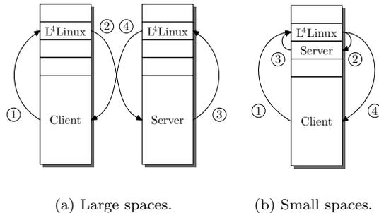
Figure 5: Pipe based communication on an L<sup>4</sup>Linux system for applications running in large versus small spaces.
