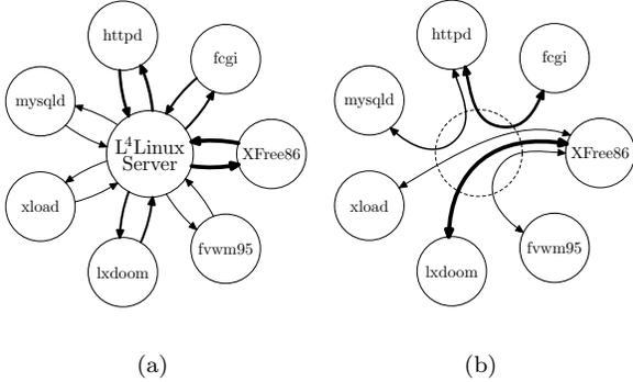
Figure 10: In L<sup>4</sup>Linux it seems that all tasks communicate with the Linux server only (a). As (b) shows, however, they actually communicate in small groups.
