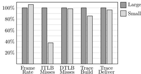
Figure 8: A comparison of LxDoom performance measurements when running the X server in either a large or a small space. Numbers are normalized to executing it in a large space.
