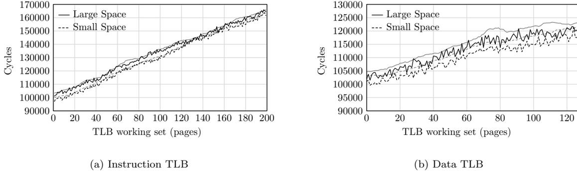
Figure 7: Processing time for thttpd and FastCGI request for different FastCGI server TLB working set sizes. The black lines show the minimum number of cycles seen (i.e., best case), while the gray lines show the average.
