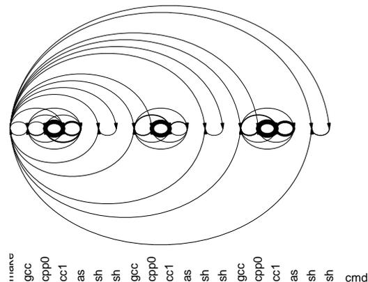
Figure 9: Compiling three source files in the Linux kernel tree. Switches always happens in clockwise fashion. The line width indicates the number of times a certain switch occurs (the width being a logarithmic function on the number of switches).
